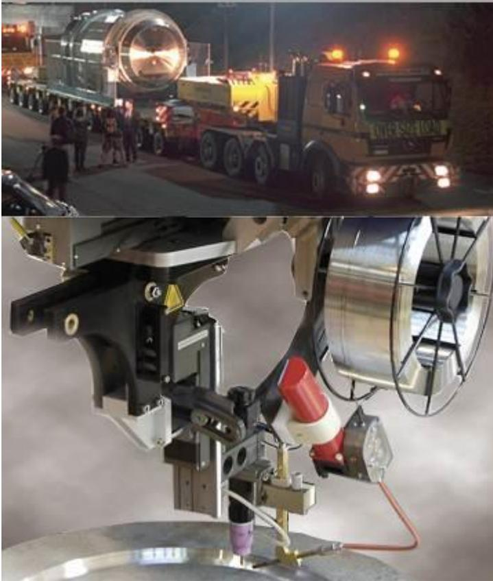
*Fig. 22: Canister seal welding for recycling of used fuel and nuclear waste disposal*
