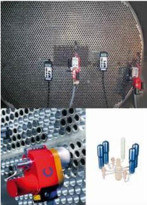
*Fig. 15: Steam generator tube-to-tube sheet welding using two welding heads*
