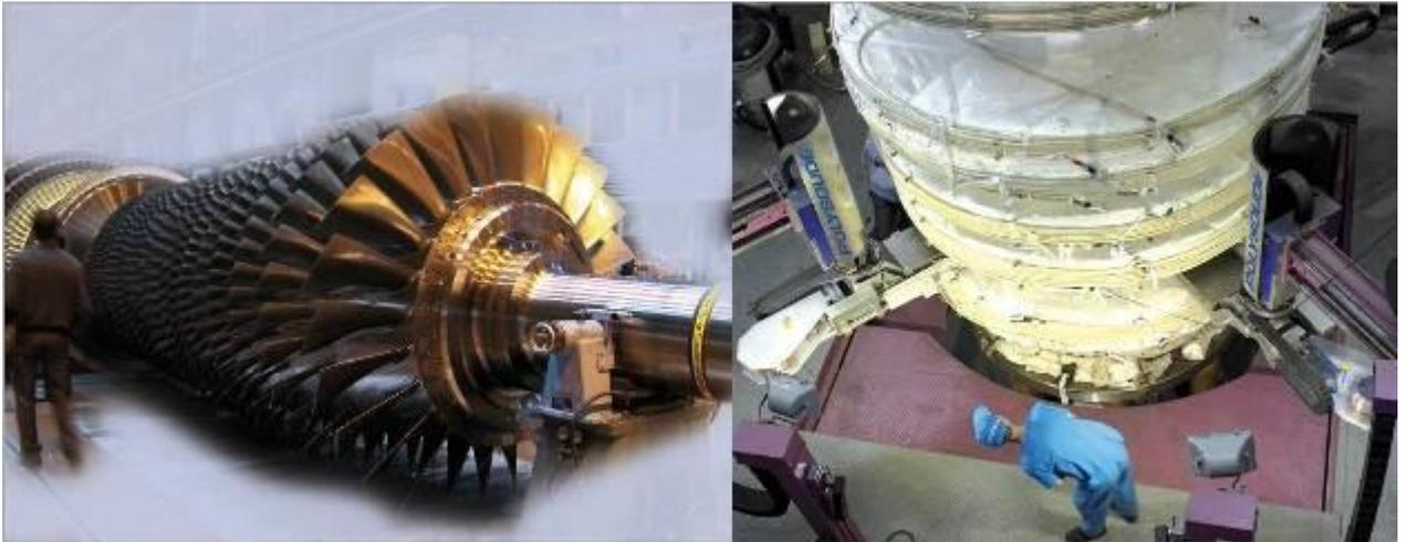
*Fig. 19: TIG welding station for joining vertically super positioned rotor segments*
