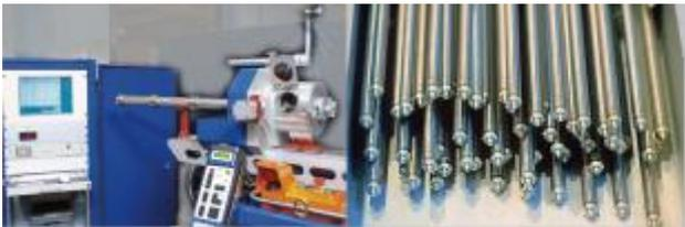
*Fig. 7: Precision vacuum welding lathe for high alloy steel end caps*
