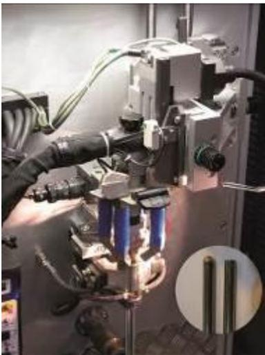
*Fig. 8: End cap welding with magnetic arc deviation*
