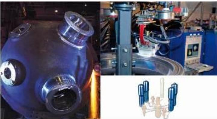
*Fig. 12: Preparation of a heterogeneous joint of the safe-end (buttering operation)*
