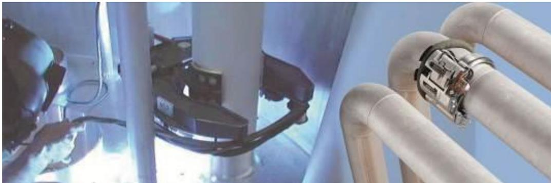
*Fig. 4: Complex piping systems in a uranium enrichment facility welded using a Polycar 30 low profile open carriage-type welding head*
