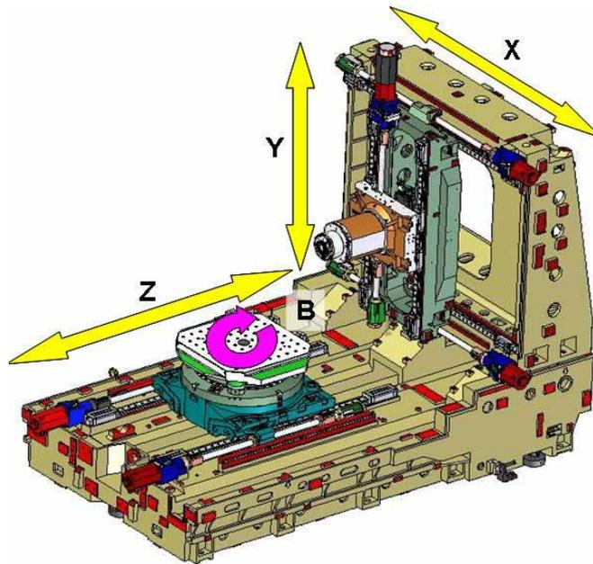
Fig. 2. Axis structure
