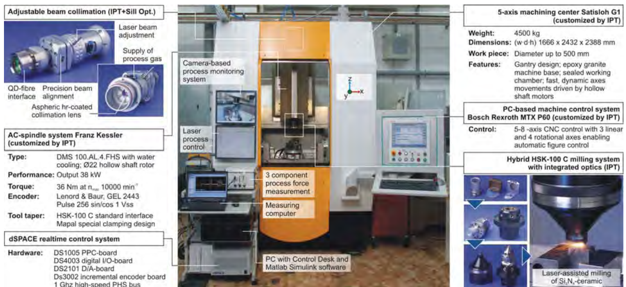
Fig. 9: Integration of all system and control components into a hybrid 5-axis machining center for laser-assisted machining of Si 3 N 4 ; technical specifications of the spindle system and the machining center (laser source and fiber-coupling are not shown in the picture)
